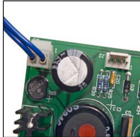
Transformer plug position J5
