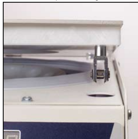
Lid latch to lid (correct position aligned to side)
