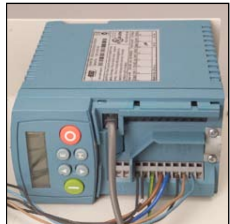
Mains connection to Inverter
