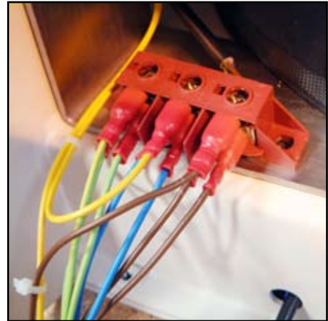
Mains plug for compressor fan and heater
