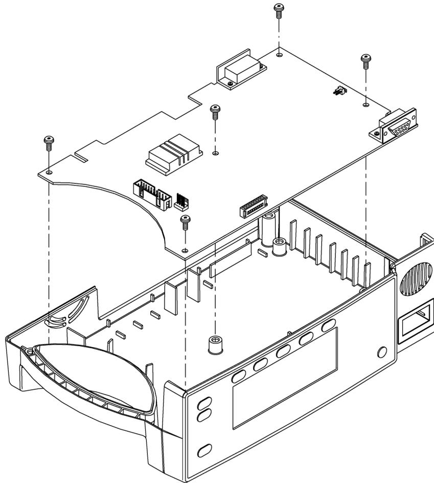
**Figure 12: User Interface PCB**
