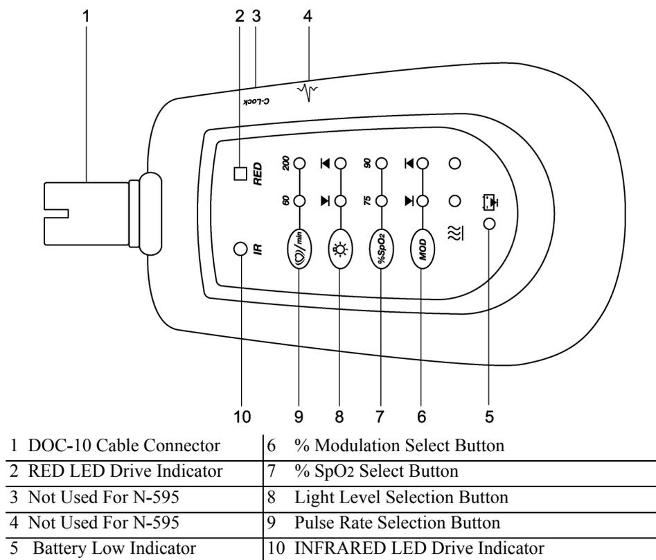
**Figure 3: SRC-MAX OxiMAX Oximetry Tester**
