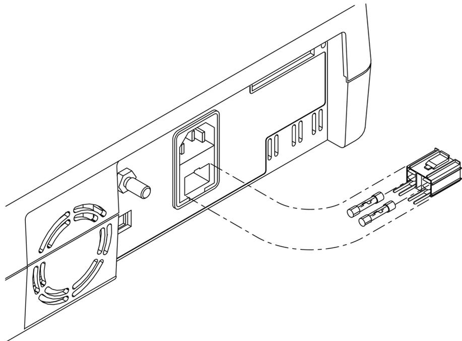
**Figure 4: Fuse Removal**
