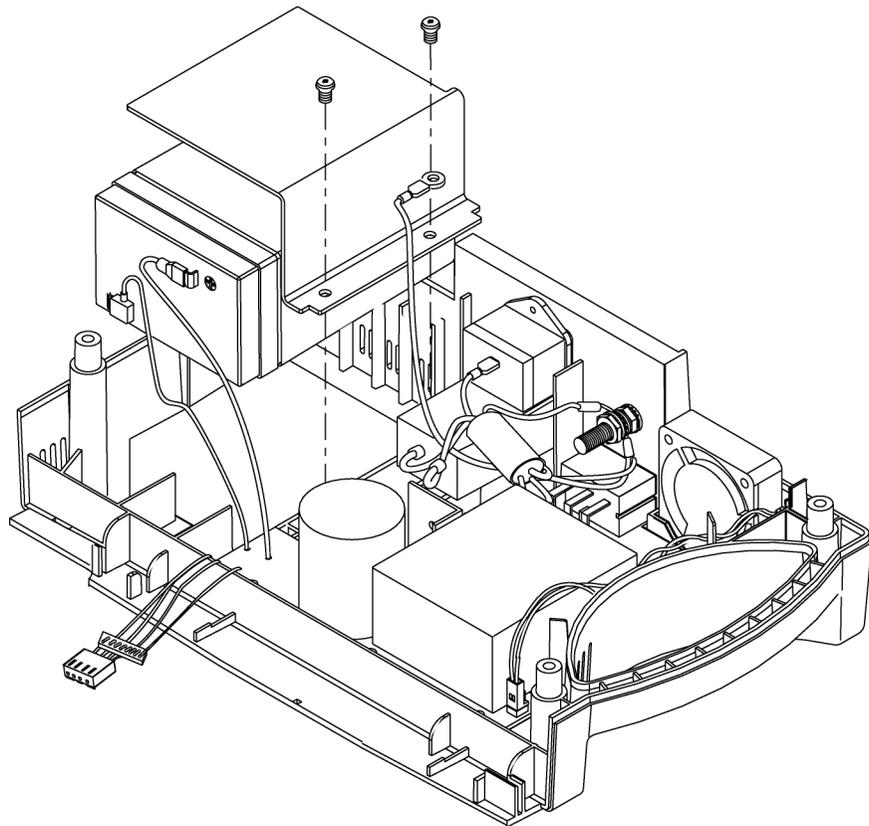
**Figure 7: Removing the Battery**
