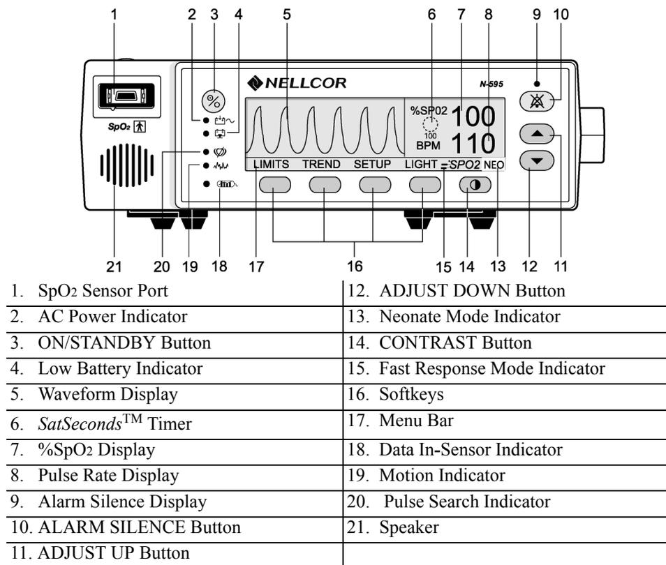
Figure 1: N-595 Front Panel
