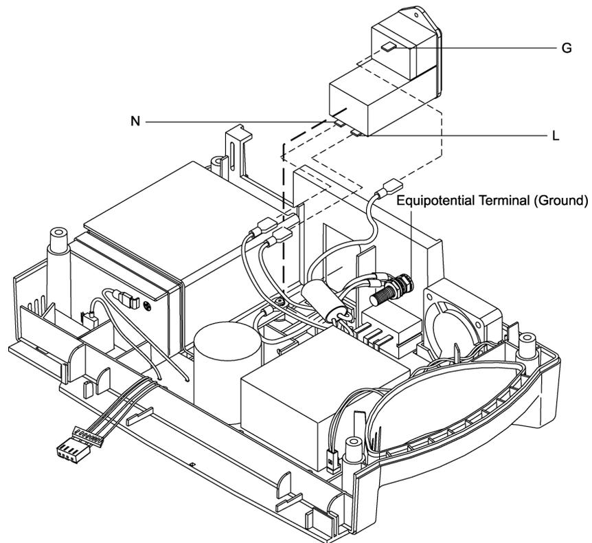
**Figure 8: Power Entry Module**
