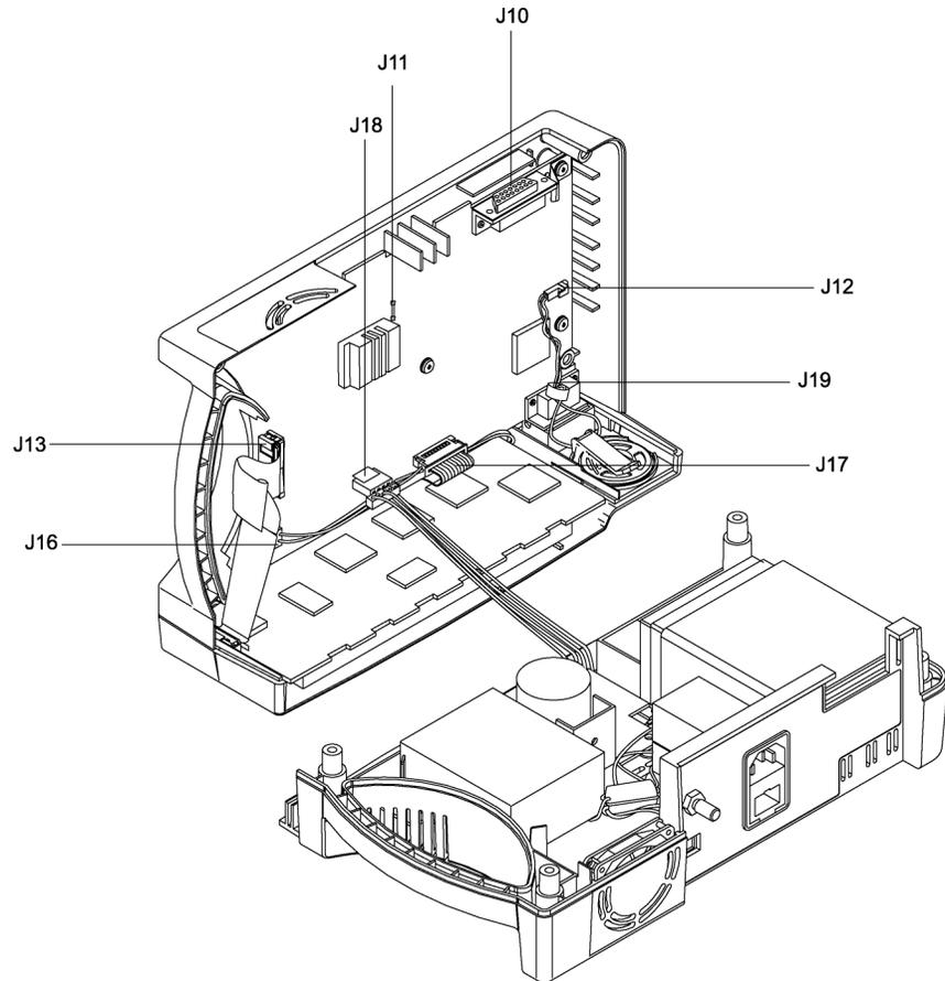
**Figure 6: Separating Case Halves**
