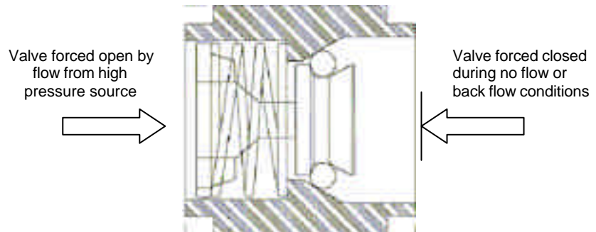
Fig 3-5, Section Through Check Valve
